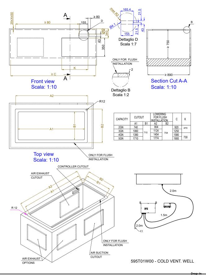
Drop-in refrigerated well, ventilated (5 GN container capacity)
